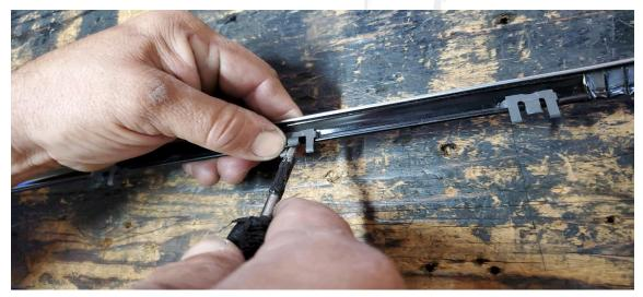
Once the scrapers are fully installed, slightly bend them outward for easier placement into the door. Line them up and press them into place.
