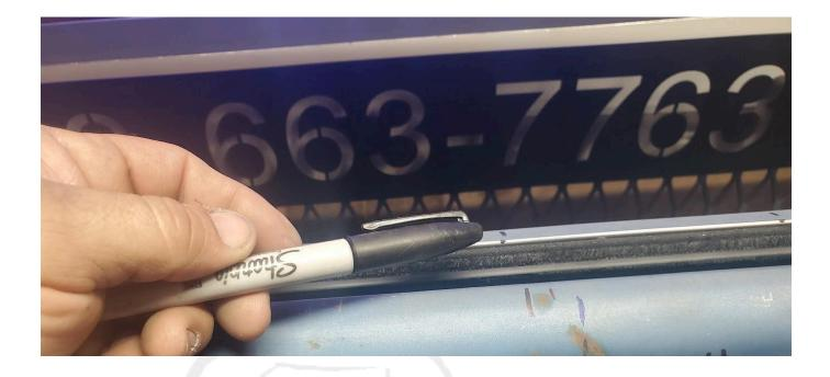
• Pre-bend each clip to ensure proper alignment when inserted into the scraper. Insert the clips, ensuring they staple toward each other for a secure fit. Position the scraper on the door, line up the sharpie marks, and press the clips in place. For areas without clip slots, use urethane or weatherstrip adhesive to secure the scraper. Repeat the process for both sides.
