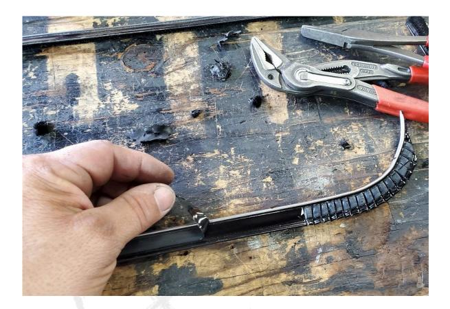
• Once the scraper is bent to the desired shape, flatten the slotted areas with pliers. Mark the original slots on the door using a sharpie for clip placement. Align the scraper and mark the corresponding points on it.
