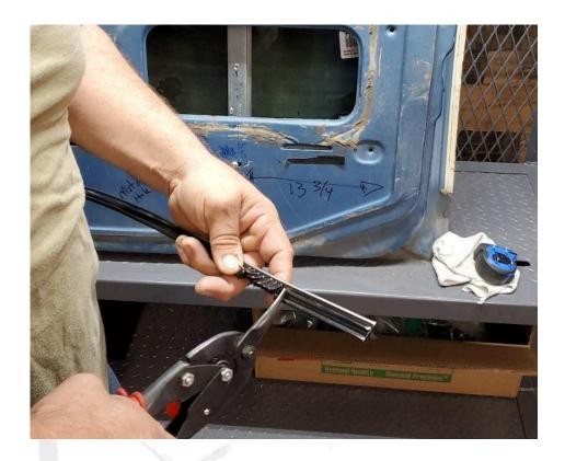
• As you bend, ensure the scraper aligns evenly with the outside and inside profiles. Trim any excess and angle cut the edges for a smooth fit against the run channel. Continue adjusting the bend as needed to match the body line.
